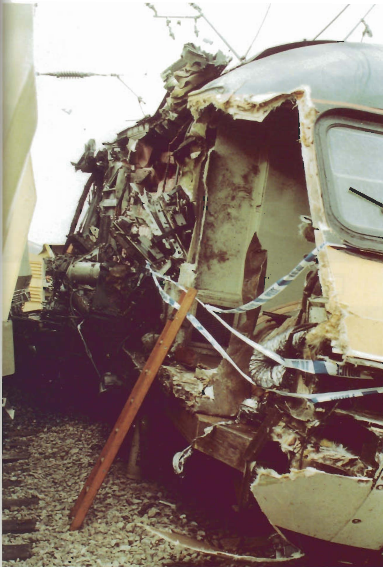
Damage to Power Car 43173 (Right Hand Side)
