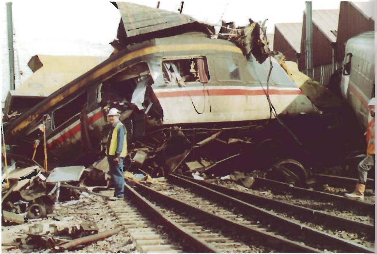
Damage to Coach G (main picture) and to Coach F (RHS)
