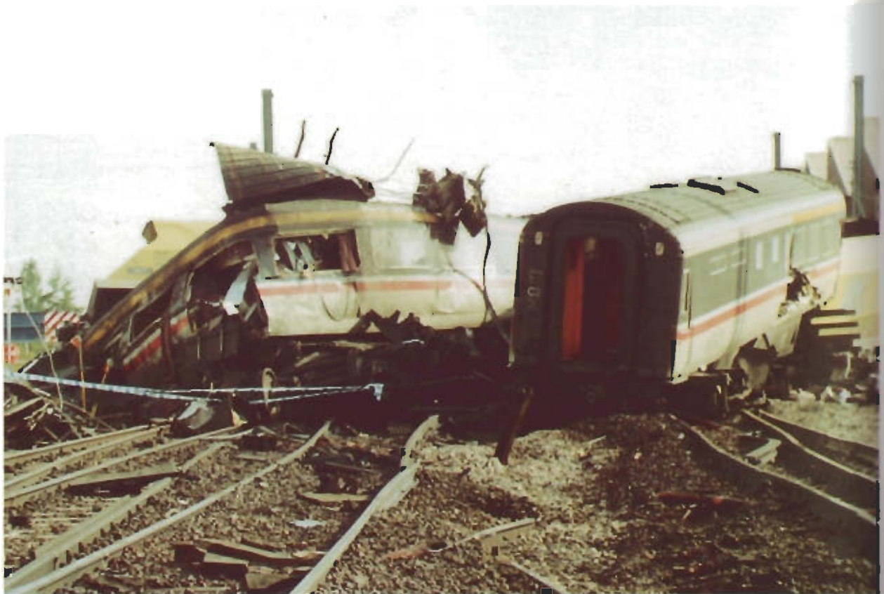
Damage to Coach G with Freight Wagon Coupler to left of picture / Coach F to the right
